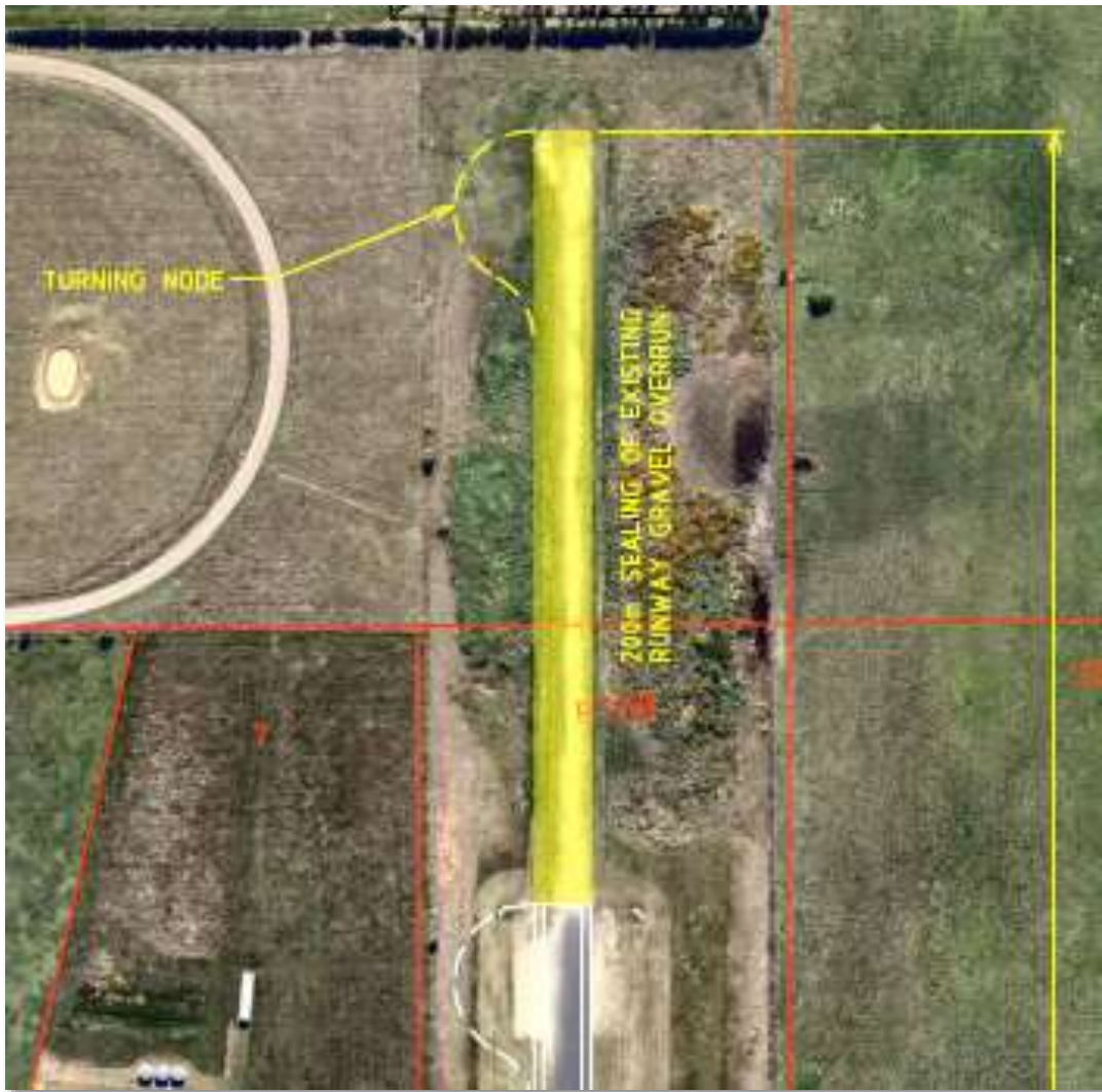
Figure 4: Runway 18/36 Northern overrun seal
