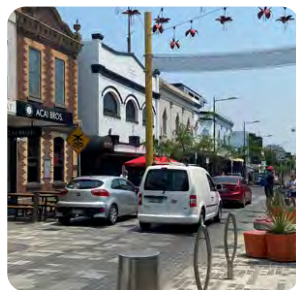
Raised tables and changed surface texture alerts drivers to pedestrian priority
