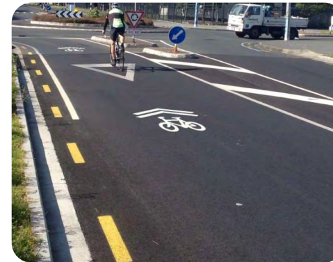
'Sharrows' are appropriate on low-speed local streets where cyclists and drivers must coexist in the same lane
